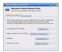
**2** Click **Pattern Recognition Tool** to open the Neural Network Pattern Recognition Tool. (You can also use the command nprtool.)
