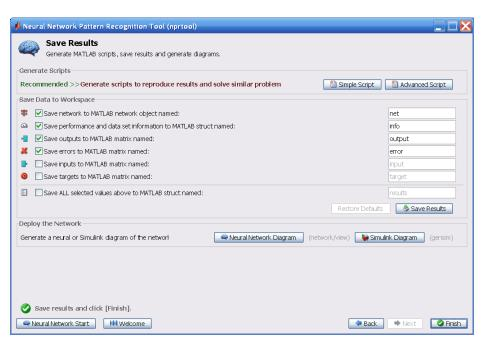
14 Use this panel to generate a MATLAB function or Simulink diagram for simulating your neural network. You can use the generated code or diagram to better understand how your neural network computes outputs from inputs or deploy the network with MATLAB Compiler tools and other MATLAB code generation tools.
