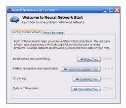
**2** Click **Fitting Tool** to open the Neural Network Fitting Tool. (You can also use the command nftool.)
